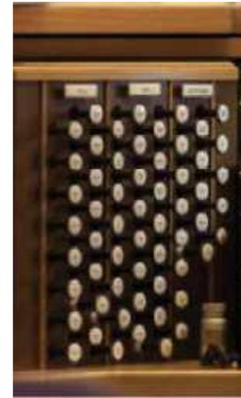
A: One of two control panels for the 1971 Schanz organ. The 'stops' electronically control the sounds from groups of the over 4000 organ pipes near the front plus three locations in the balcony.
